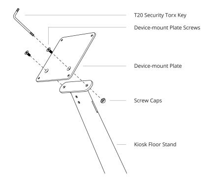
2 Install device to mounting plate.
